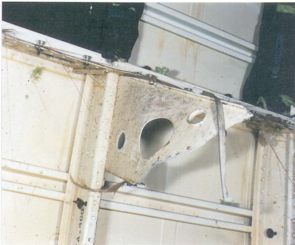
Appendix 3, figure 20 - Floor beam at station 460 (area I)
