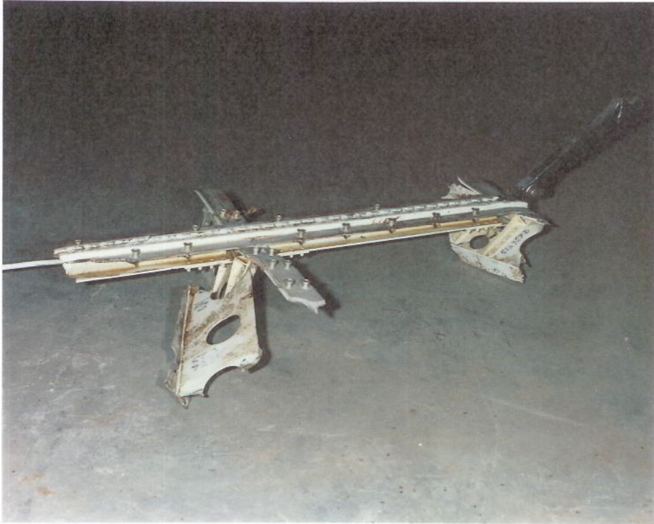
Appendix 3, figure 17 - Seat track at station 727D (area III)
