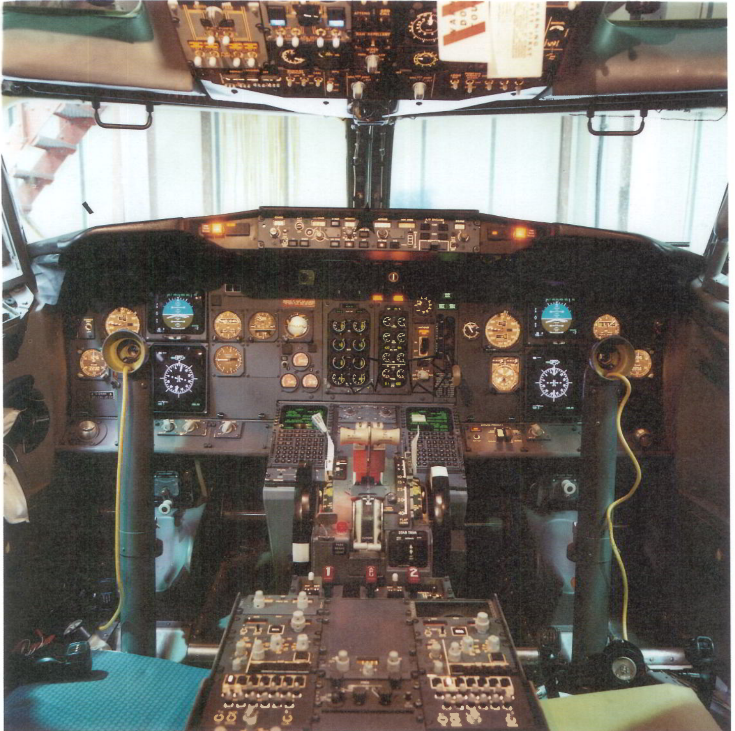
FIG. 2: SHOWING SOLID-STATE ELECTRONIC ENGINE INSTRUMENT SYSTEM (EIS), AS FITTED TO G-OBME, WITH VIBRATION INDICATORS ARROWED
