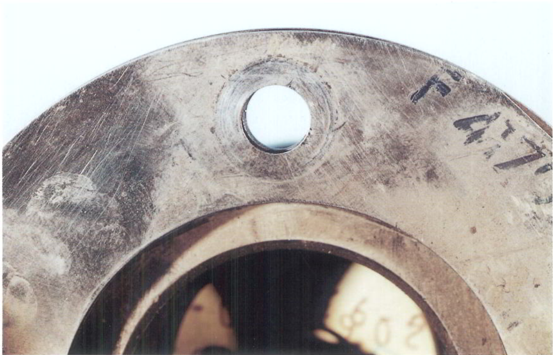
Plate 1a Undamaged bolt hole through flexor plate stack from Thomas Coupling
