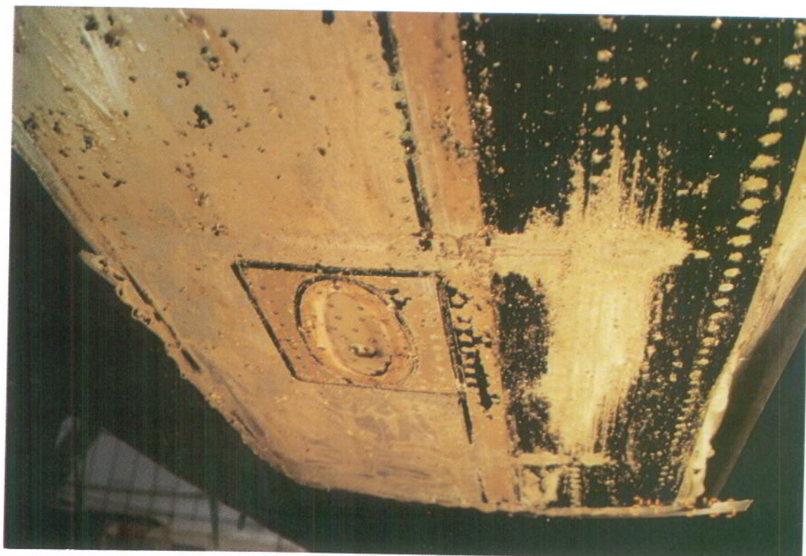
View on underside of G-BRYJ looking forward. Note "touch runway" switch mounting plate to the left of the centreline
