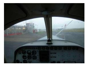
Figure 7 View from cabin of ZK-KAY Note - view from the pilot's eye position (left and lower) is compromised by the windscreen strut and engine cowling
