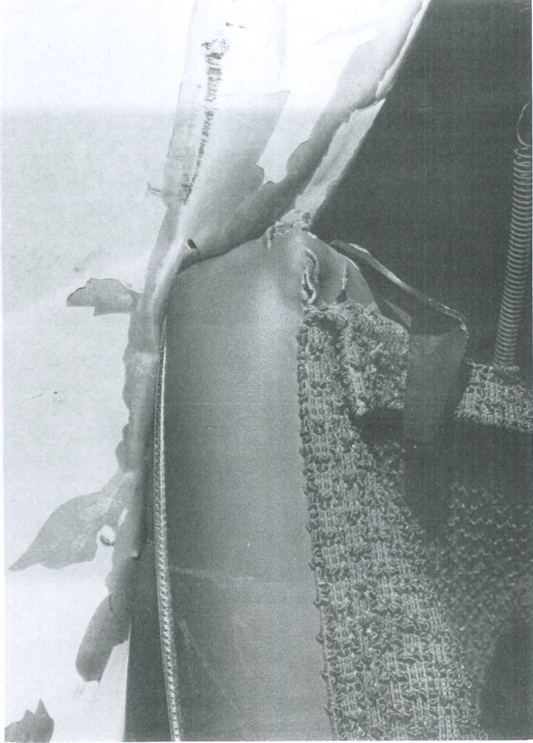
Fig.12 Seat corner fitting stabilator leading edge damage
