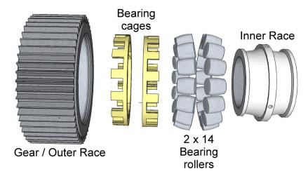
**Figure 8** Planet gear configuration
