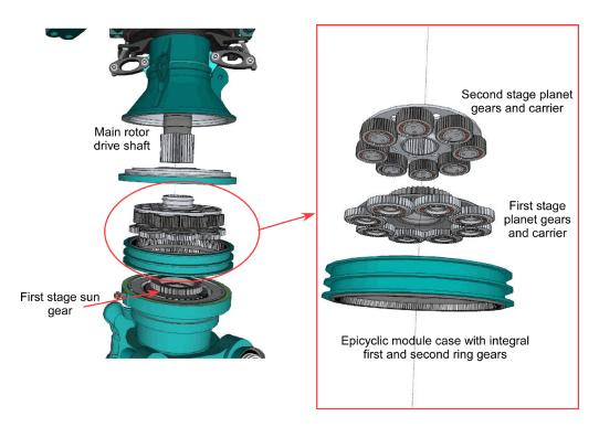
**Figure 7**Layout of the epicyclic reduction gearbox
