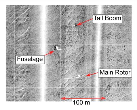
**Figure 2** Sidescan sonar picture of main wreckage items
