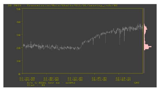
**Figure G-1**G-REDL HUMS lower planetary bearings Band Energy
