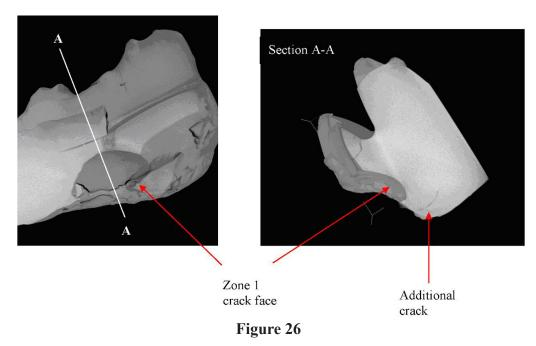
Tomographic image of section of 9-tooth section fracture face
