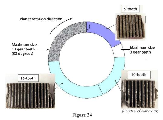
Relative position of recovered second stage gear sections
