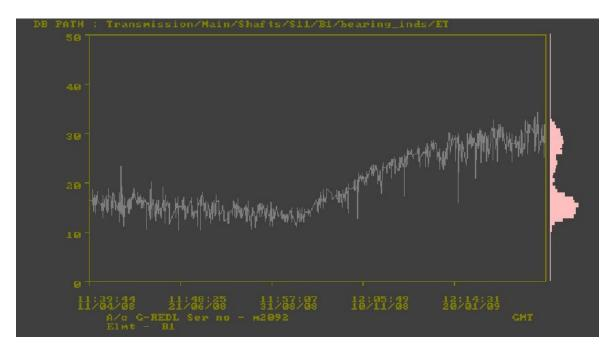
**Figure G-2**G-REDL HUMS lower planetary bearings Tonal Energy
