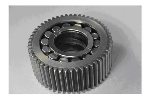
**Figure 22**Complete undamaged gear, for reference
