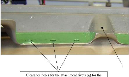
Clearance holes for the attachment rivets (g) for the magnetic elements (e)
