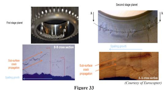
Spalled gears exhibiting cracking within the carburised layer
