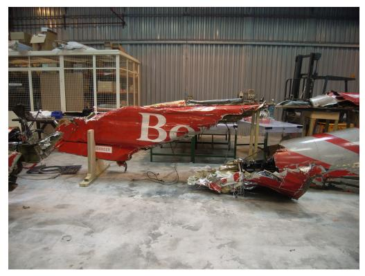
**Figure 19** Helicopter tail boom after recovery
