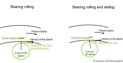
**Figure 32**Bearing rolling and sliding
