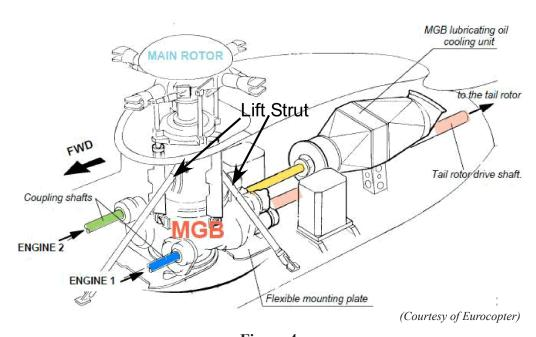
**Figure 4** Transmission layout diagram
