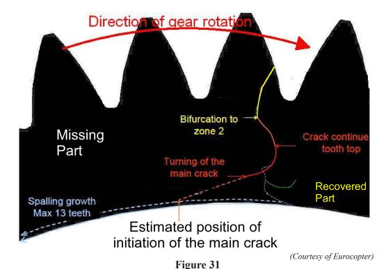
Stress model prediction of crack growth
