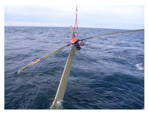
**Figure 3** Main rotor head recovery
