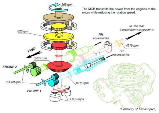
**Figure 6**Main rotor gearbox internal configuration
