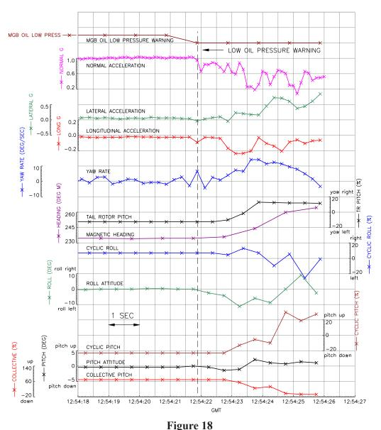
Flight control inputs and helicopter response
