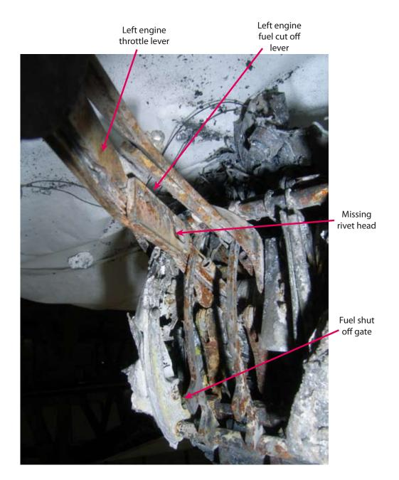
**Figure 7** Throttle quadrant post-impact on VP-BGE
