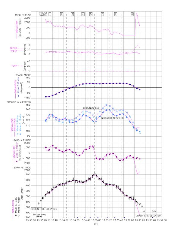
**Figure D-1** Simulation results of accident flight – flaps up
