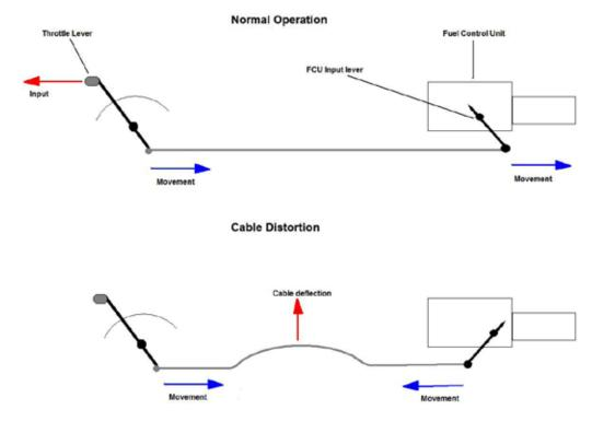
**Figure 16** The effect of engine control cable distortion
