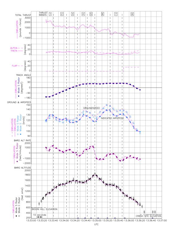
Figure D-3 Simulation results of accident flight – flaps 0-15
