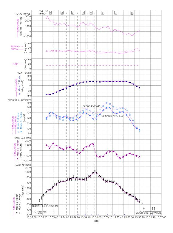
**Figure D-2** Simulation results of accident flight – flaps 15
