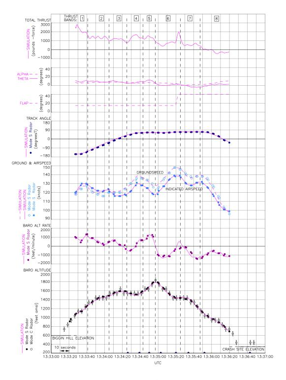
**Figure D-4** Simulation results of accident flight – flaps 15-40
