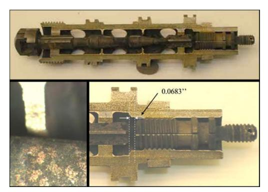
**Figure 11** Sectioned left engine FCU metering valve
