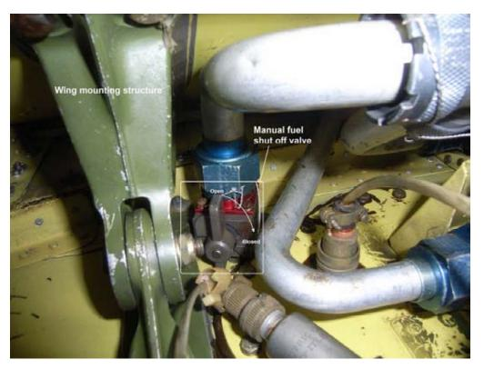
**Figure 9** Manual fuel shut-off valve
