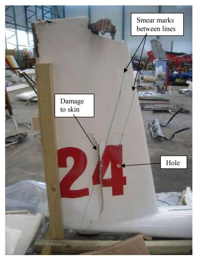
**Figure 22** Damage to the glider's fin
