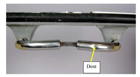
Figure 17 Canopy locking bracket on G-BYXR
