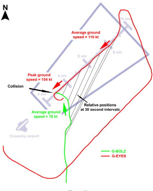
**Figure 10** Tracks and speeds of G-BOLZ and G-EYES
