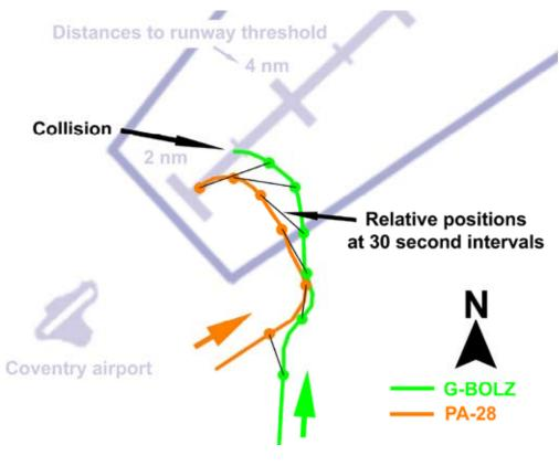
**Figure 9** Separation between G-BOLZ and the PA-28
