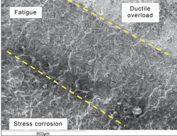
Figure 4 Fracture surface map
