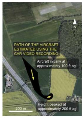
**Figure 3** Path of the aircraft estimated from analysis of the car video recording
