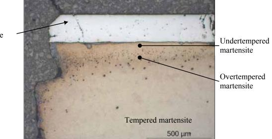
Figure 6 Fracture surface metallurgy
