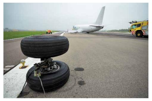
Figure 1 View of aircraft and detached section of lower left MLG
