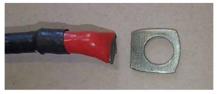
**Figure 3** Failed terminal lug on the end of the phase 'A' generator ground cable
