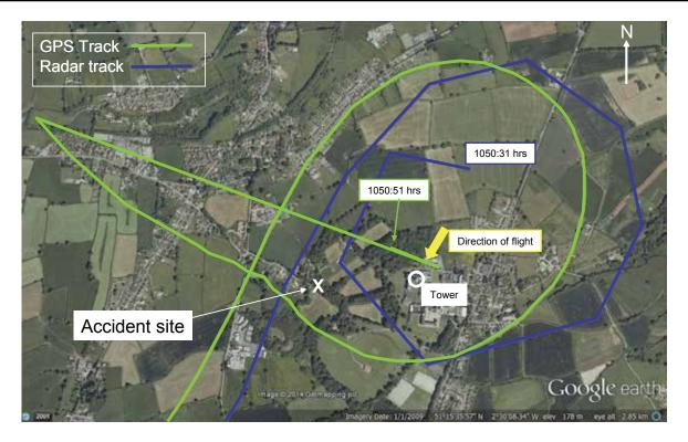
**Figure 3** GPS and radar tracks for the final stages of the flight
