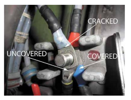
Figure 7 Cracked terminal lug from ground cable at T191 stud on G-GDFB's No 2 engine
