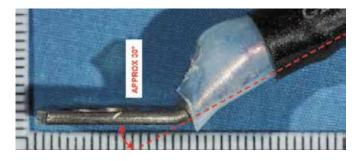
Figure 12 30° upwards bend of cracked G-CELF ground lug
