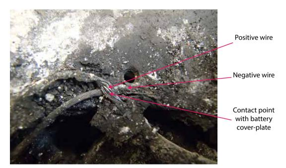
Figure 2 Crossed and pinched ELT battery wires
