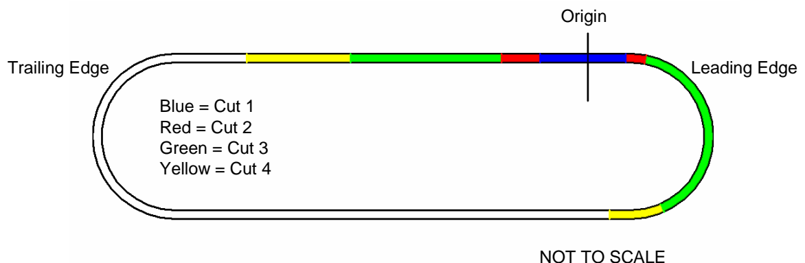
Figure 1. Cross section through spar showing crack positions.
