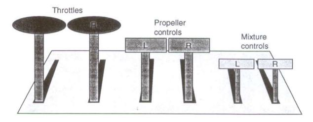
Figure 2: Conventional engine control layout
