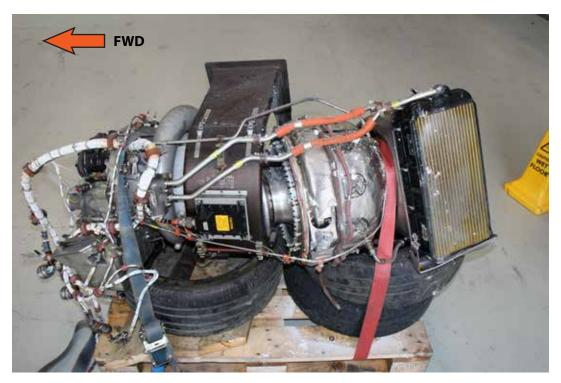
**Figure 6** Underside of APU after removal, showing extent of the damage
