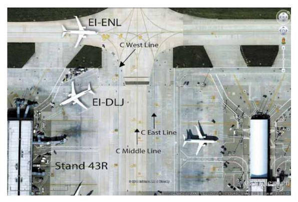
**Figure 3** Relative position of EI-ENL when EI-DLJ push back commenced (composite image)
