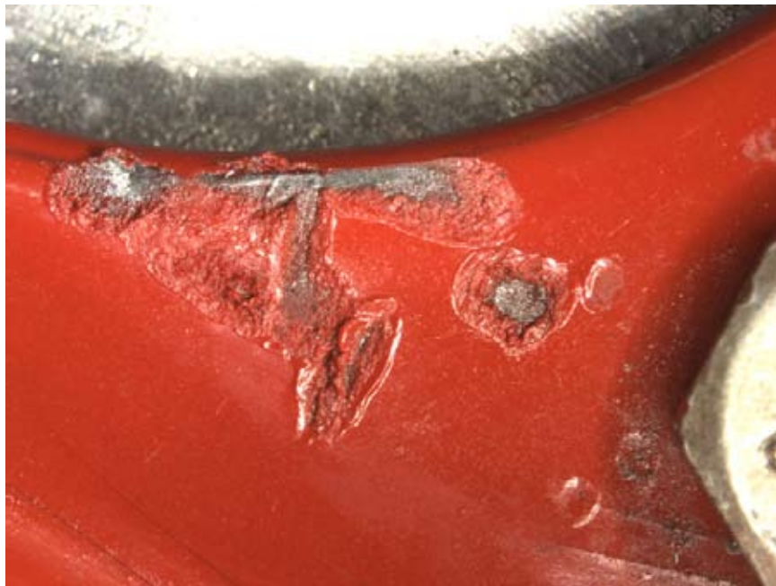
Figure 9 Close up of Figure 8 showing witness marks probably made by the end of the pip-pin
