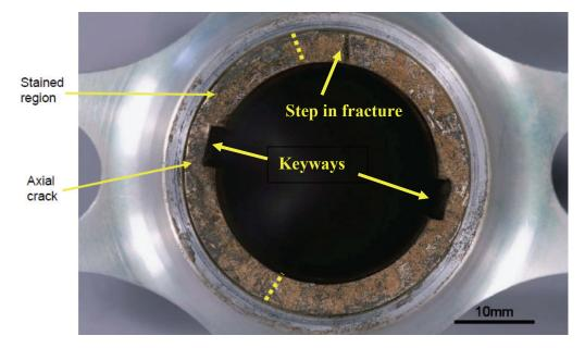
Figure 3 View of bearing fracture face
