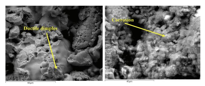
**Figure 5a** Fracture surface in clean area
