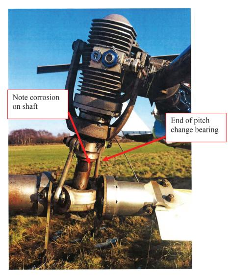
**Figure 1** Tail rotor assembly after the accident
