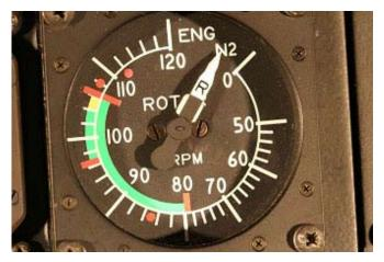
The two N2 pointers are below the NR pointer in this photograph of the gauge at rest. Note the tail of the NR pointer.
