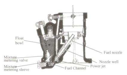
Figure 3 Section through carburettor
