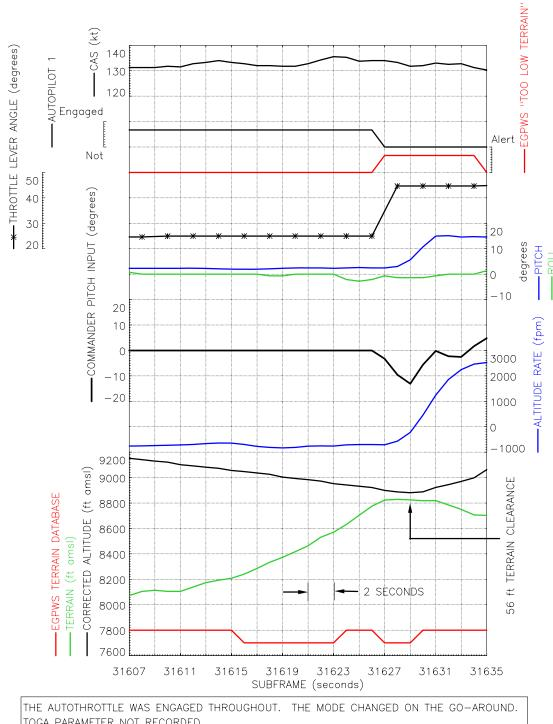
TOGA PARAMETER NOT RECORDED THE GEAR AND FLAPS WERE IN LANDING CONFIGURATION THROUGHOUT THIS PERIOD
