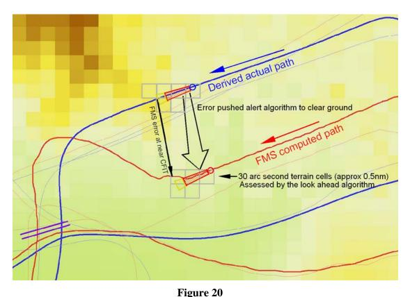
FLTA - Honeywell alert envelopes in relation to the navigation error
