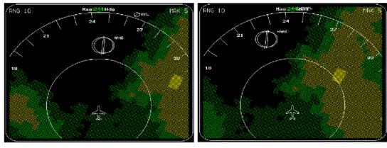
With FMS Position Error Approximately 2.6 NM cross-track error
