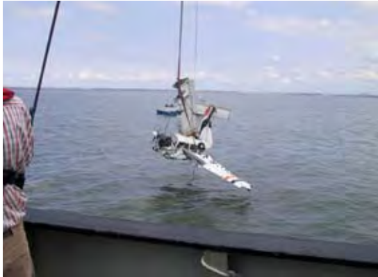
Wreckage recovery from the sea in good weather conditions
