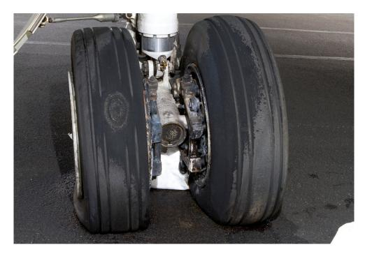
Figure 3 Fire damage to the left main gear tyres and brakes (view looking forward); flat spot on left tyre
