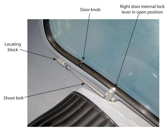
Figure 4 Right door operating mechanism
