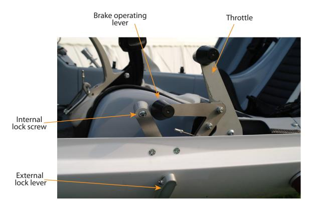
Figure 5 Throttle restricted by internal lock lever.
