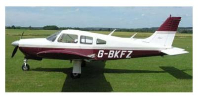
**Figure 1** PA-28R-200, G-BKFZ, with a two-bladed propeller fitted
