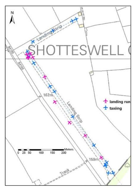
Figure 1 Landing and subsequent taxiing at Shotteswell airstrip prior to accident flight
