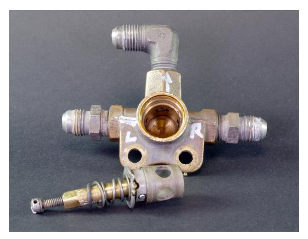
Figure 2 Fuel selector valve (valve cap removed)
