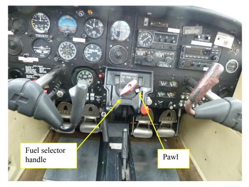
**Figure 1** Fuel selector handle in the OFF position
