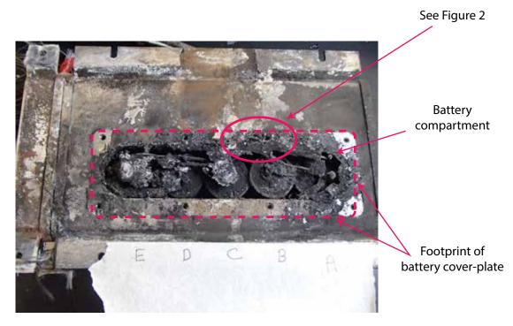
**Figure 1** ELT case with battery cover-plate removed; tops of battery cells visible
