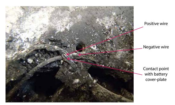
Figure 2 Crossed and pinched ELT battery wires
