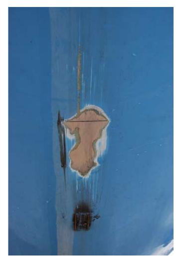
**Figure 1** Damage to the underside of the aircraft tail
