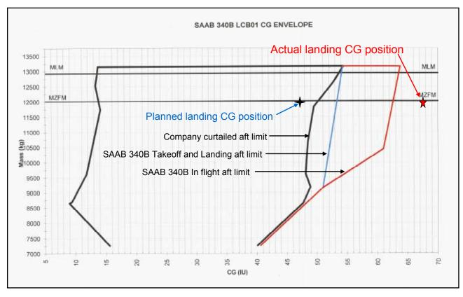
Figure 2 SAAB 340B CG position limits for takeoff, landing and flight
