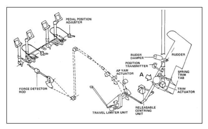
**Figure 1**ATR 72 Rudder control system
