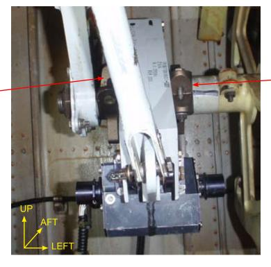
Left hand cam (correctly installed)
