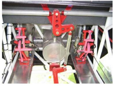
Figure 4 Rudder pedals with pedal extensions (pink) fitted
