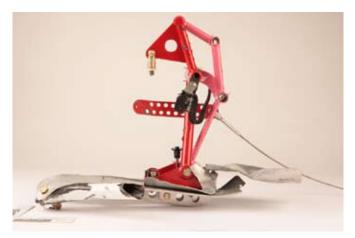
Figure 5 Right rudder pedal with extension
