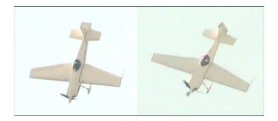
Figure 11 The point of recovery in practice manoeuvre (left) compared to the equivalent point during the accident manoeuvre
