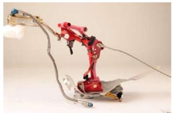
**Figure 6** Left rudder pedal with extension
