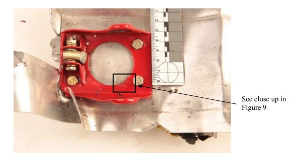
Figure 8 Base plate for left rudder pedal
