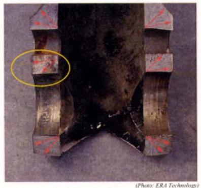
Figure 3 Initiation and propagation of the various ligament fractures. Corroded fracture (circled) characteristics are different from others
