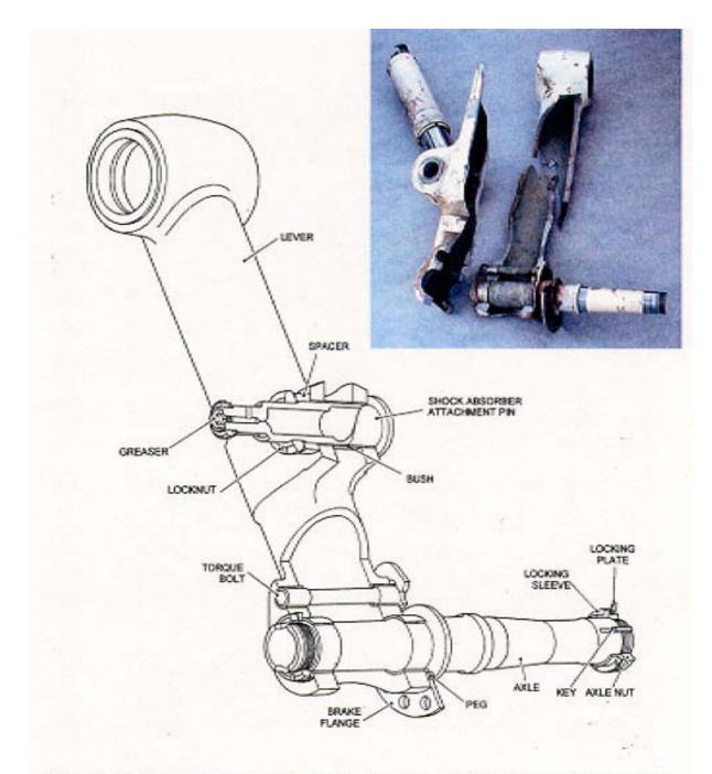
(Note: for clarity, the lever is shown sectioned at lower end. By coincidence, the failure occurred along the plane of section, as seen in the inset photograph.)
