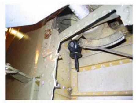
Figure 2 (screwdriver, as discovered, jammed on the aft elevator quadrant)
