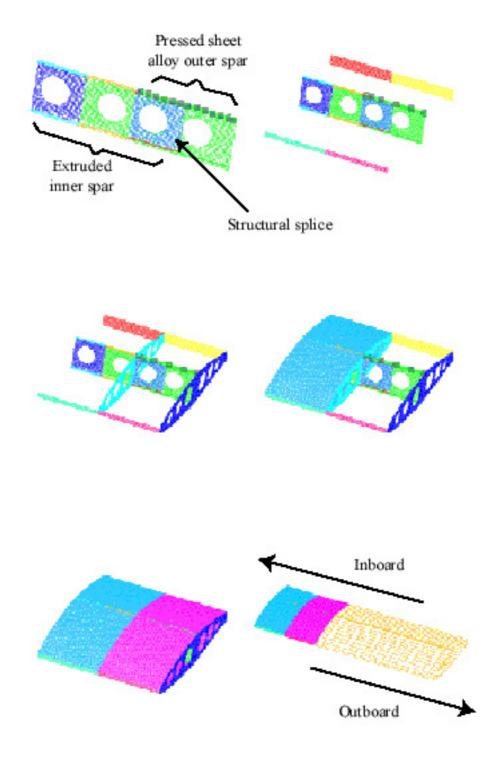
Build-up of structural components for Finite Element (FE) model
