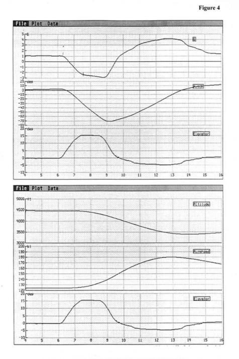
Calculated aircraft response - 15° stabilator angle for 3 seconds
