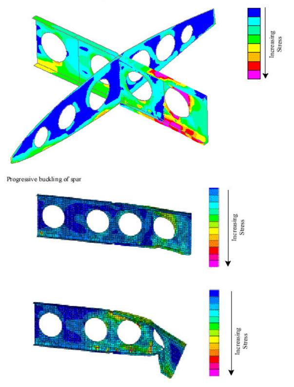
Finite Element Analysis Visualisation of Internal Structure
