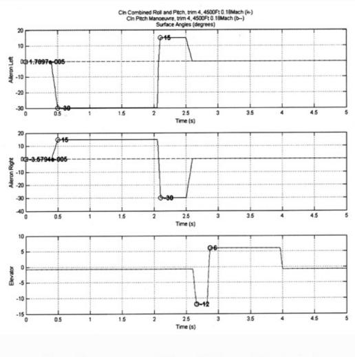
Control input sequence which resulted in very high wing loads in a downwards direction
