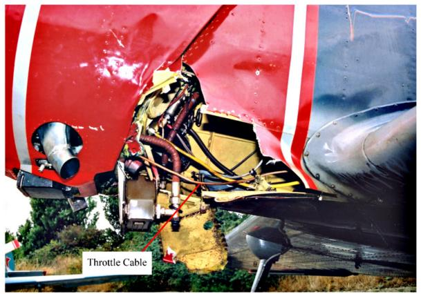
The oil cooler fairing detached and a portion of a fuselage main longeron was torn out, separating the associated engine mount from the airframe. The throttle cable sheath had been permanently deformed forward of its fuselage attachment, displacing the inner cable and thus opening the throttle.
