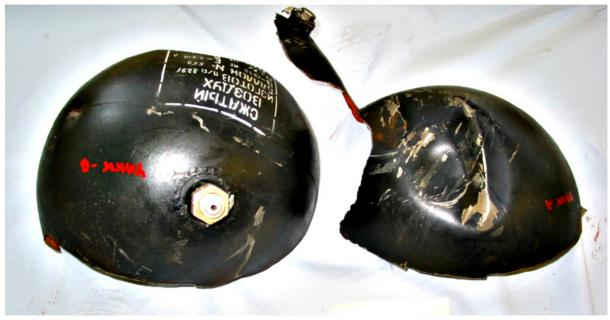
The internal surfaces of both were found to be covered completely with rust deposits, with numerous areas of deep corrosion pitting (Figures 7 and 8).
