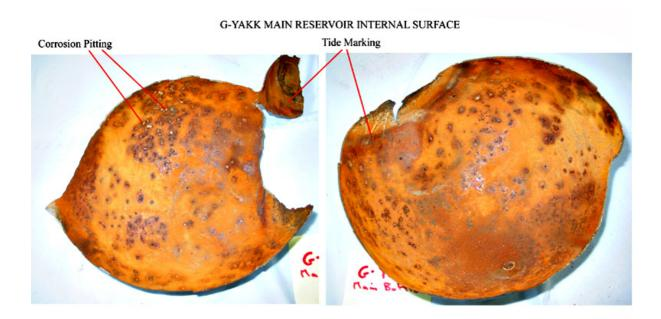
A number of corrosion pits had extended almost to the exterior surface; this was clearly evident in the case of a number of pits that had been bisected by the fracture (Figure 9).
