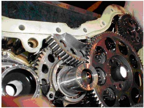
Figure 3 Failed intermediate gear from G-PUMS
