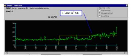
Figure 4: Two EuroARMS data plots, showing threshold breaches
