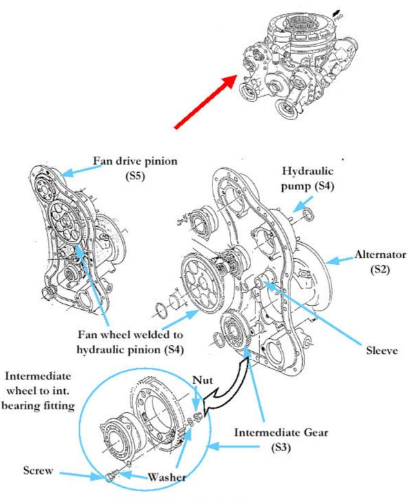
Figure 1 Details of left hand accessory module
