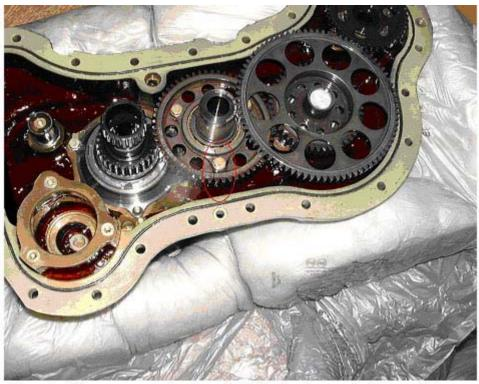
Figure 2: LH accessory gearbox module from G-JSAR, showing cracked intermediate gear
