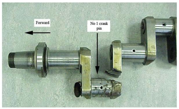
Figure 3 - Fractured crankshaft
