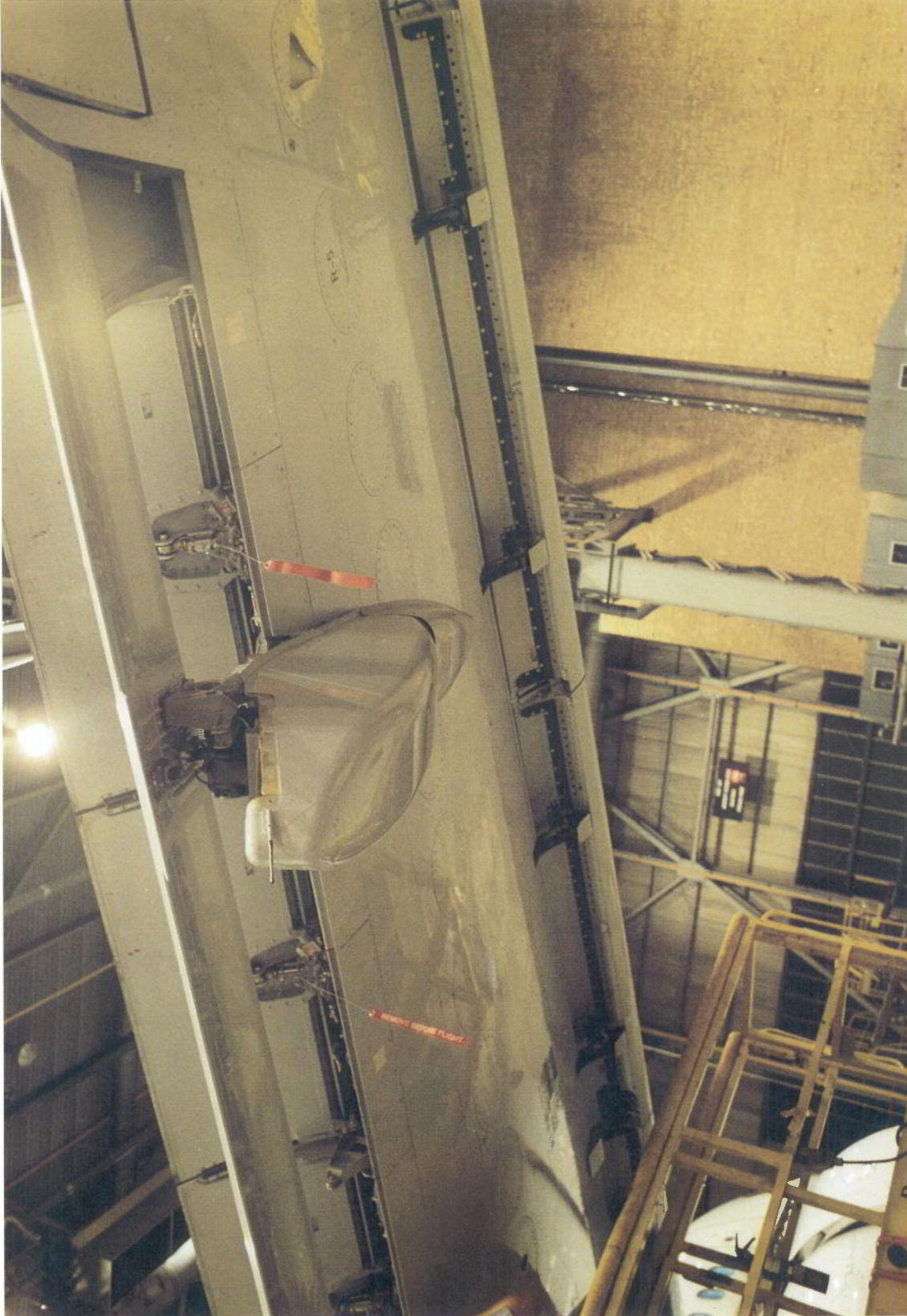
VIEW ON TRAILING EDGE SHOWING FLAPS AND SPOILERS EXTENDED, AND COLLARS AND FLAGS IN POSITION
