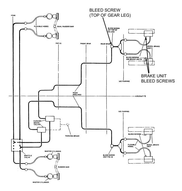
**Figure 3** Diagram of the brake system
