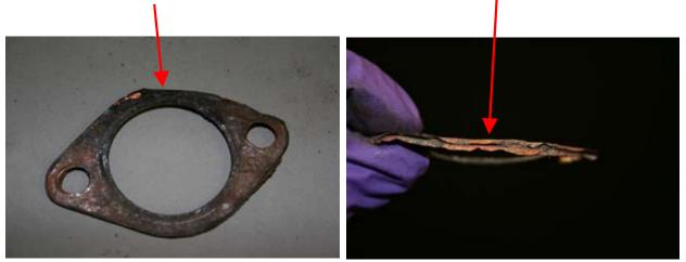
Figures 2 & 3 Exhaust gaskets removed from the accident aircraft
