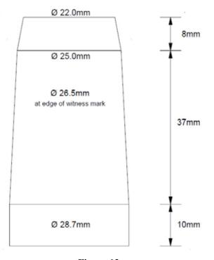
Figure 12 Dimensions of the bevel bolts
