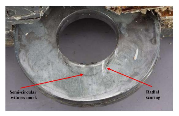
**Figure 20** Mechanical damage on upper surface of the left hand (centre) lug
