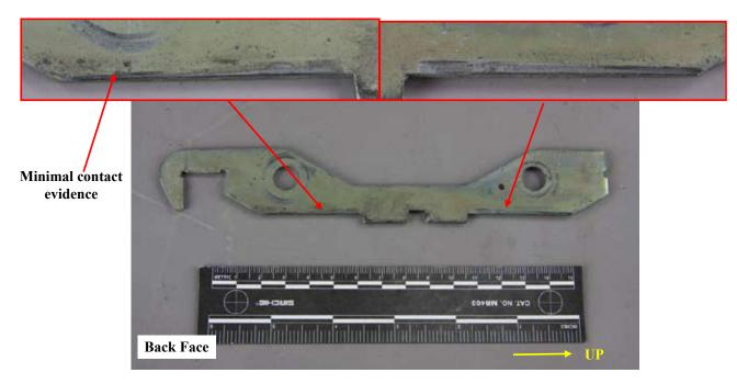
Figure 14 Wear marks on back face of aft guide plate
