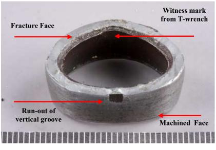
Figure 10 Fractured section of lower bevel bolt
