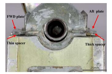
Figure 13 Difference in stand-off between forward and aft guide plates
