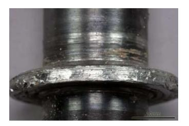
Figure 18 Mechanical damage observed on surface of collar
