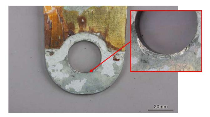
Figure 19 Mechanical damage observed on upper right hand lug
