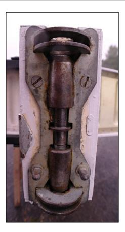
**Figure: 3 (a)** Wing Main Fitting, bevel bolts fully retracted
