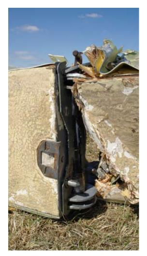
**Figure 9** Wing main fitting in correct orientation
