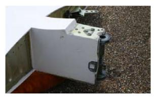
**Figure: 1 (a)** Right wing root with Wing Main Fitting
