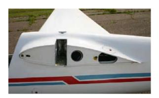
Figure: 1(b) Fuselage spar cut-out, right wing installed; access hole visible in top of fuselage
