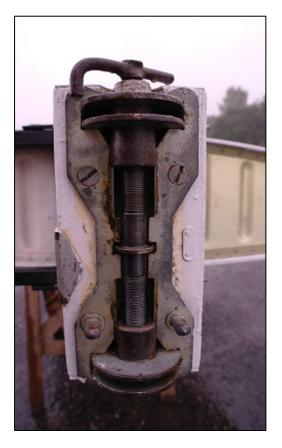
**Figure: 3(b)** Wing Main Fitting, bevel bolts fully expanded and T-wrench inserted
