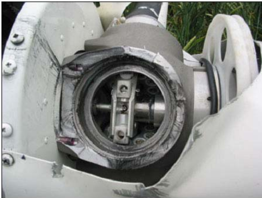
Figure 1: Propeller hub showing fractured blade arm
