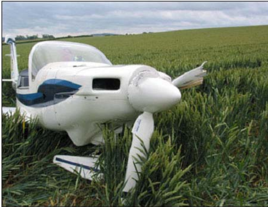
Figure 2: General view of propeller damage
