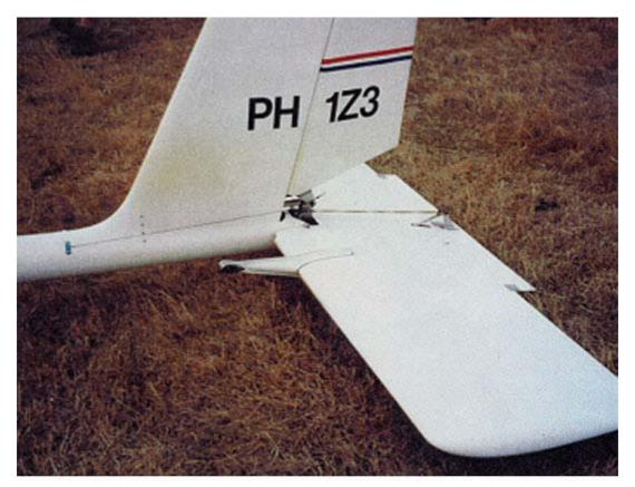
Figure 6 Sirocco tailplane with mass balance modification incorporated
