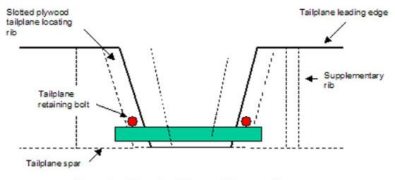
Figure 3 - Schematic of Sirocco tailplane attachment
