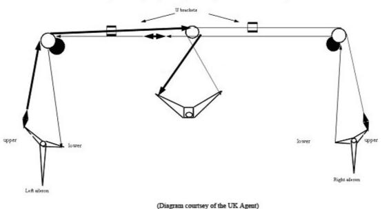
Diagram of aileron control system cable routing indicating cable crossover between aileron yoke and pulleys at top of cockpit windscreen centre pole
